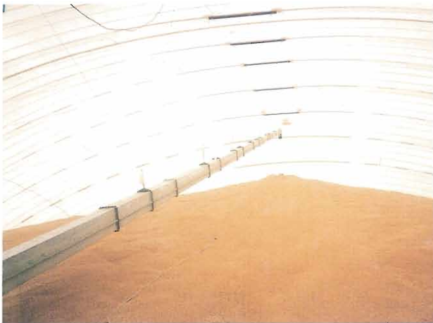
252' Diameter x 63' High Clear Span Featuring an elevator through the dome wall, and suspended from the inside of the dome
